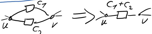
If  $c_1, c_2$  are parallel edges, the effective resistance stays if they are replaced by a single edge with the sum of conductances.
